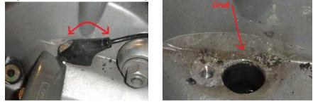
Use small screwdriver to remove front band from final drive rubber boot:
