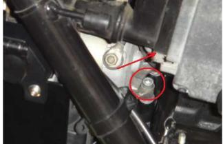
Remove center bolt (5mm) from right swing arm pivot that secures the plastic retainer for the side stand switch wiring. Remove 3 bolts (5mm) around the perimeter that secure right swing arm pivot to transmission case:
