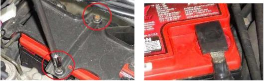
Undo negative battery terminal first to avoid risk of your tool shorting to the frame when removing the positive terminal. Undo positive battery terminal.
