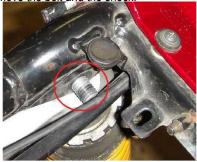
Disconnect side stand switch connector near rear brake reservoir.
