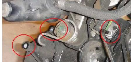
Disconnect Motronic connector by pushing metal tab at the rear of it back and lifting up the rear of the connector:
