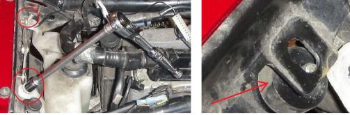
Empty coolant reservoir: Remove right "Z" rack bolts (5mm) and right peg plate bolts. (8mm)
