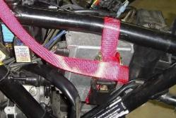
Remove 2 bolts (5mm) that hold rear of starter motor to transmission: You do not need to remove or disconnect the starter. Just make sure the transmission doesn't hit the starter when you slide the transmission back on.
