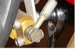
Remove nut from lower rear shock stud.
