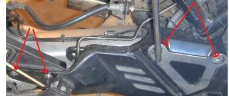
Remove 2 bolts (5mm) that hold rear master cylinder to right peg plate and bolt (4mm) that holds rear brake switch:
